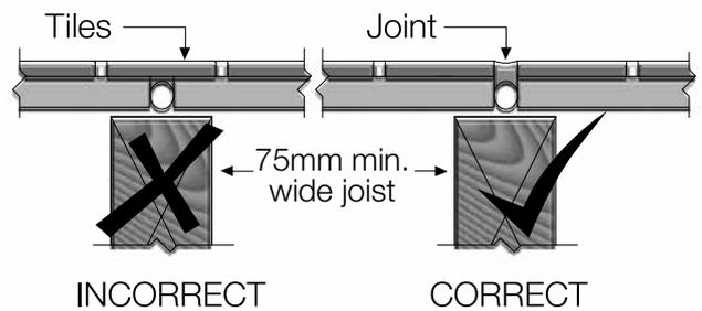
Figure 16: Waterproof deck construction
