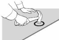
Tap carefully to avoid damage to sheets, ensuring that the sheet edges are properly supported.
