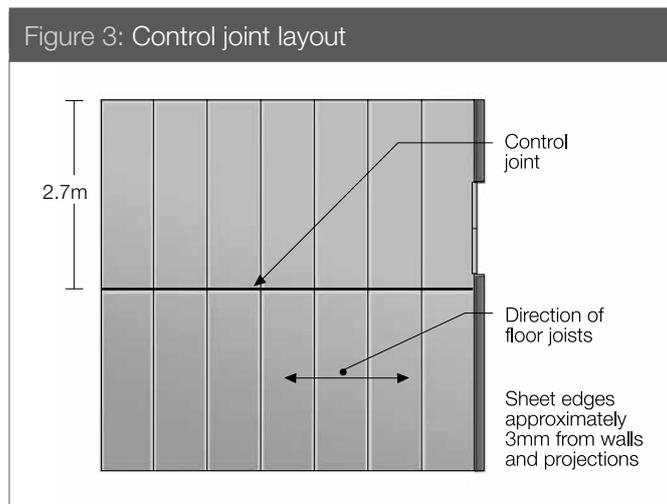
Also provide control joints where there are changes of direction, such as an L-shaped room, and at doorways where the tiled surface is carried through to the next room as shown in Figure 4.
