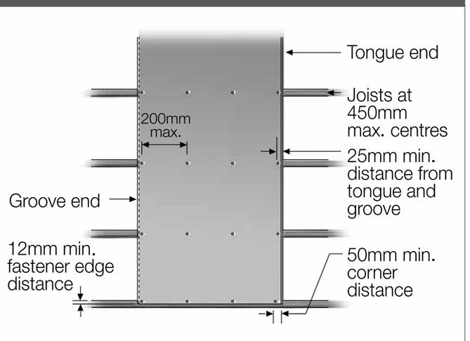
Figure 10: Fixing first panel.
