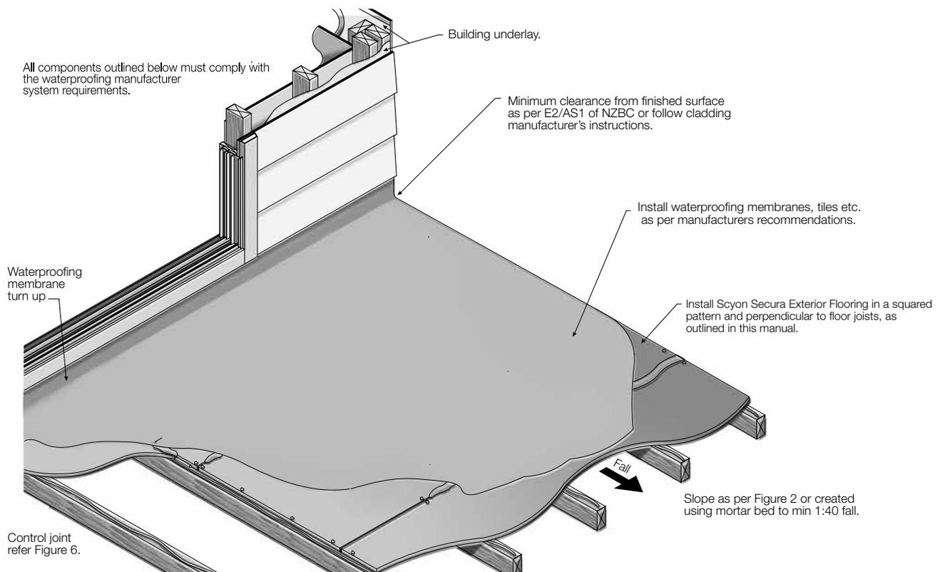
All sheet fixing must be completed as per this installation manual before the primer and waterproofing membrane is applied.
