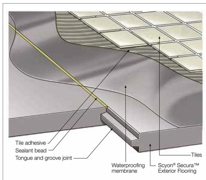
Constructing a deck/external floor involves the installation of two components;
