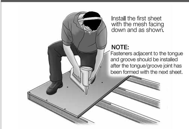
Fixings to be 50 x 2.87mm RounDrive nails at 200mm maximum centres. Refer Table 3. Alternatively a 10g x 40mm wood thread screw can be used.
