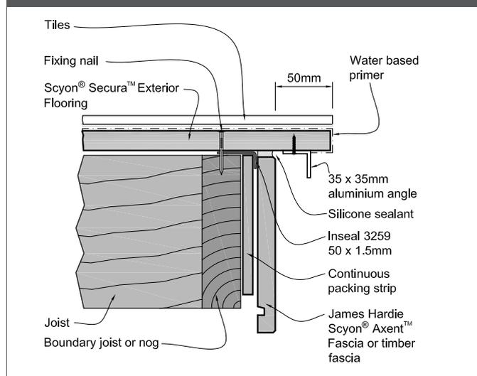
Figure 18: Wall to deck flashing
