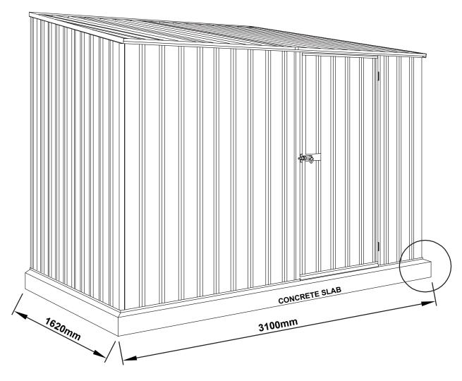
For construction in non-cyclonic areas Wind rating: N2 as per AS4055-2012
