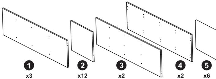
**Note:** All panels here are showing the internal view hole configurations.
