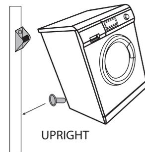
You will need to pack at the bottom spacers by the same thickness as the batten to keep the dryer upright and level.
