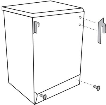
When locating the mounting brackets onto the dryer back panel, you may notice only one screw hole. If this is the case, you will need to take the other self-tapping screws to push and pierce the dryer back panel. (this will locate the hole beneath the back panel). Continue to turn the self-tapping screws until tightens. Once done, in the same manner fit the spacers to the back of the dryer.
