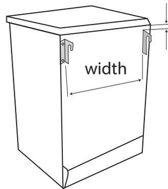
Note the measurements from the top of the dryer to the top of the dryer bracket and the distance between the dryer brackets etc.
