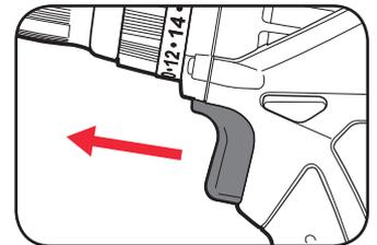
**Note:** The more the variable speed trigger is depressed, the faster the drill bit will rotate.
