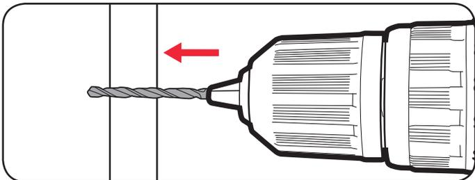
**Note:** Do not force the drill or apply side pressure to elongate the hole. Let the drill do all the work.
