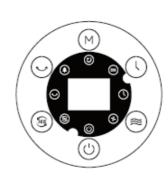
**POWER button:** Press to switch the fan on or to standby.
