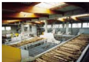
OSB line – ring knife flaker
