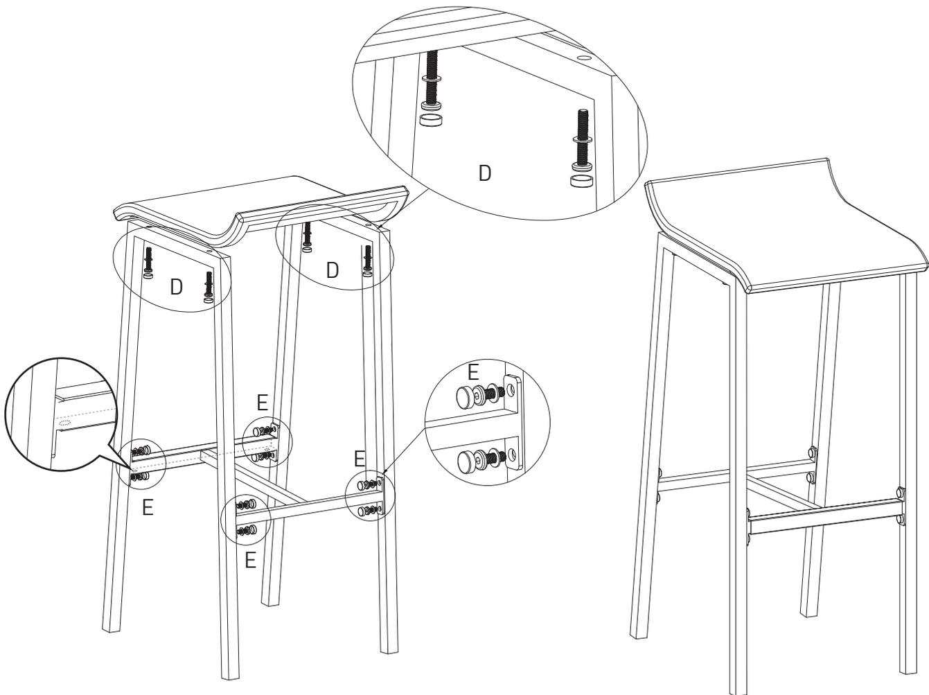
Attach support bar(B) to legs (A) with using bolts and washers(E).
