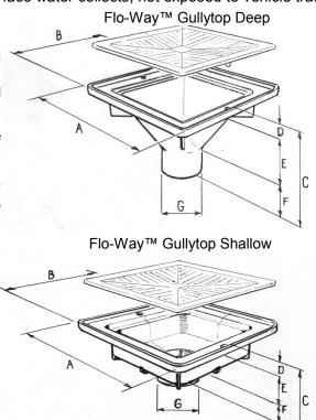
level. Use a suitable adhesive sealant such as Fuller's "Max-Seal" or equivalent to attached FLO-WAY™ to pipes. (Solvent cement will not act as an adhesive on FLO-WAY™).
