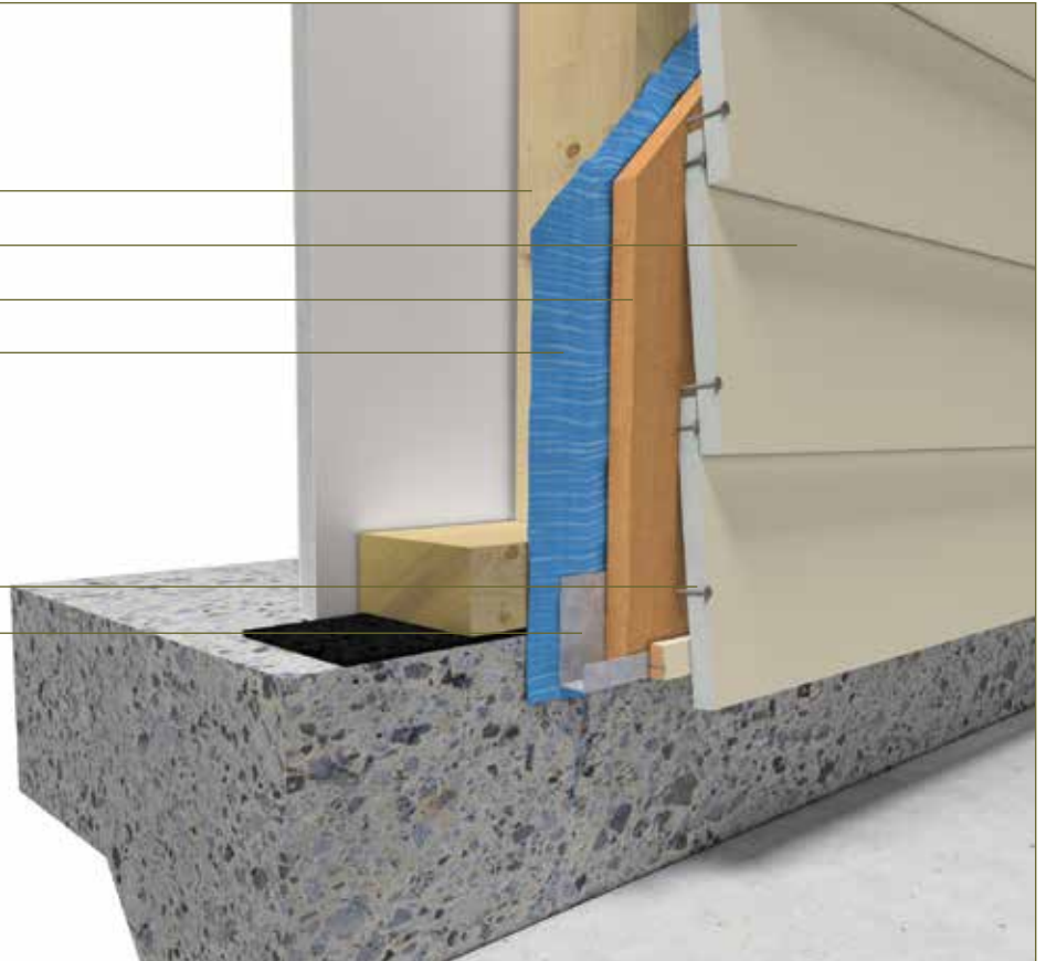
FIGURE 6 FASTENER DETAIL TIMBER FRAMING FACE FIXING SYSTEM
