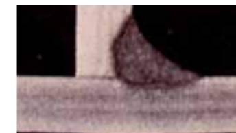
Argon: welding speed 7cm/min
