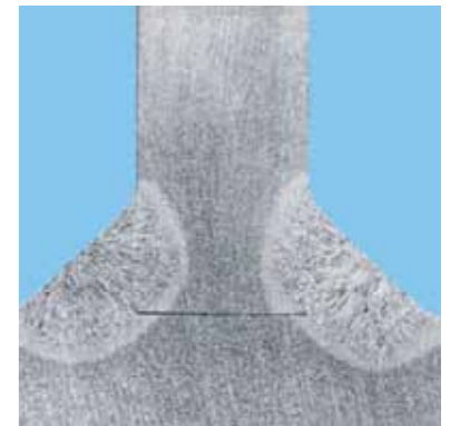
Transverse section of a fillet weld made with Coregas® He 30 showing the typical wide, trough-shaped penetration. Wire feed rate: 25m/min.
