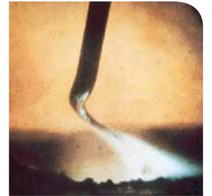
A unique feature of T.I.M.E. welding with high wire feed rates: the rotating twin arc.
