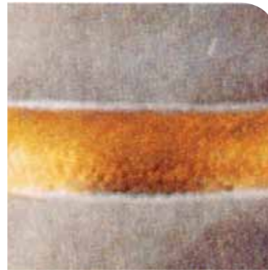
Typical yellow colouration: Titanium-stabilised CrNi steel formed with Nitrogen
