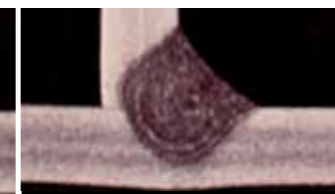
Shieldpro® 22: welding speed 11cm/min
