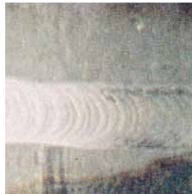
No colouration: Titanium-stabilised CrNi steel formed with Argon-Hydrogen
