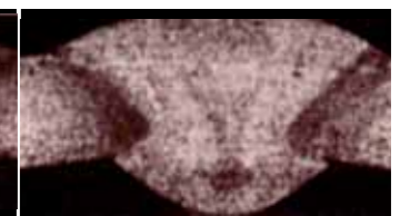
Shieldpro® He 50: 15l/min: welding speed 20cm/min
