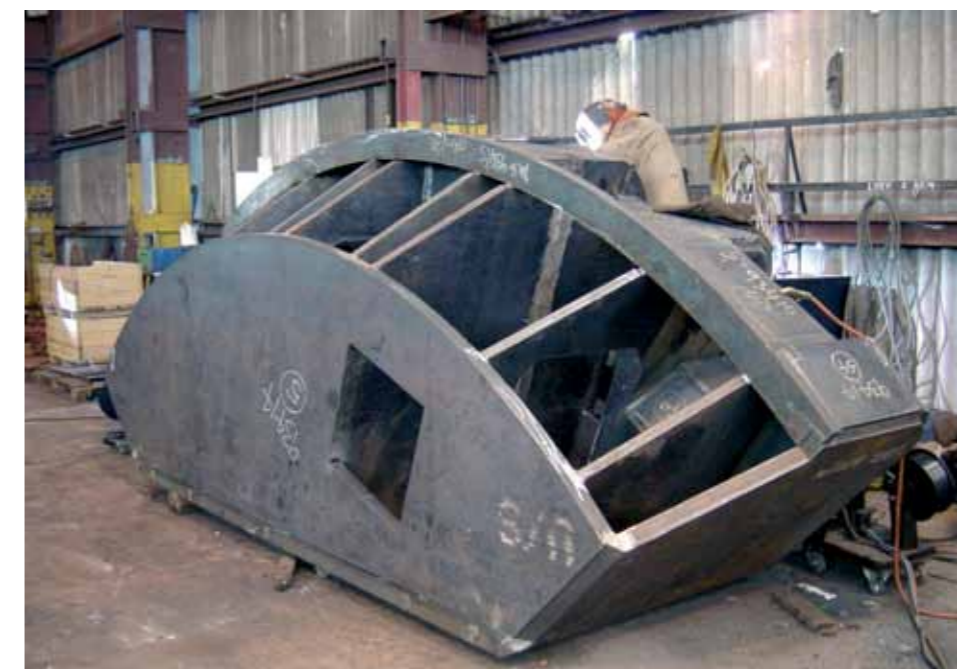
Coregas® He 30 being used with the T.I.M.E. welding process
